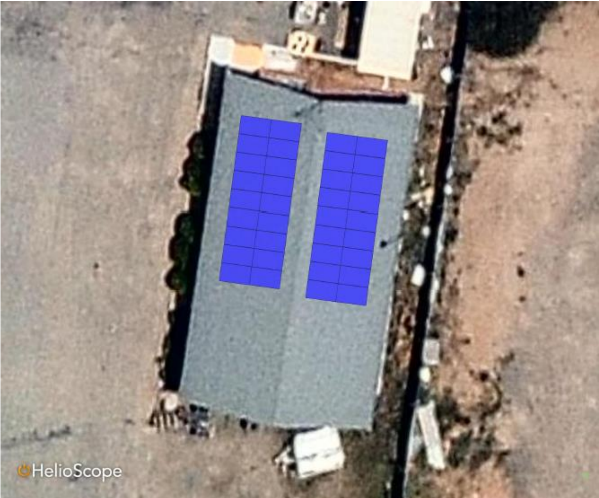
Chanter St Depot - 13.7kW - Solar PV - Roof - STC
