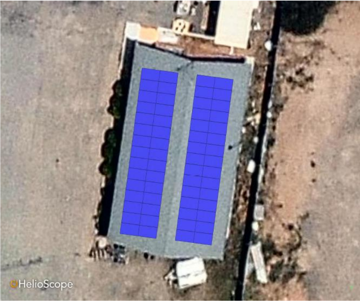
Chanter St Depot - 23kW -Solar PV + BESS - Roof - STC
