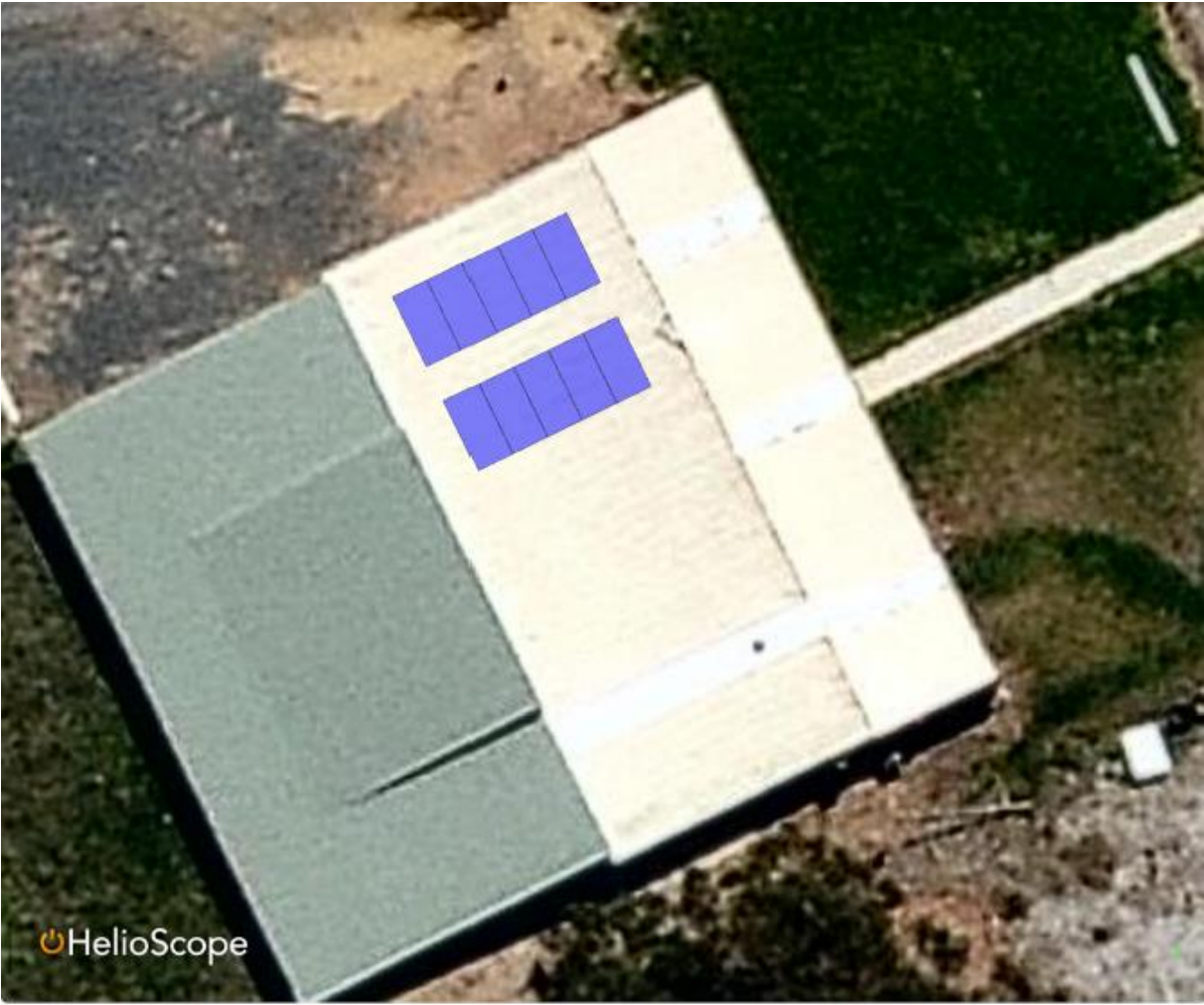
Tocumwal Aerodrome- 4.15kW- Solar PV + BESS - Roof - STC
