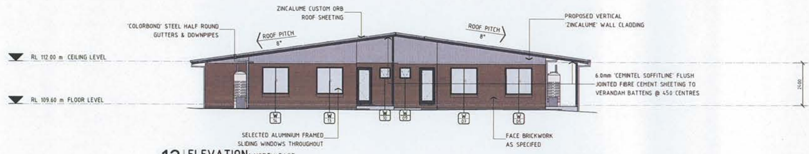
12 ELEVATION: NORTH EAST SCALE: 1 : 100 (A1)
