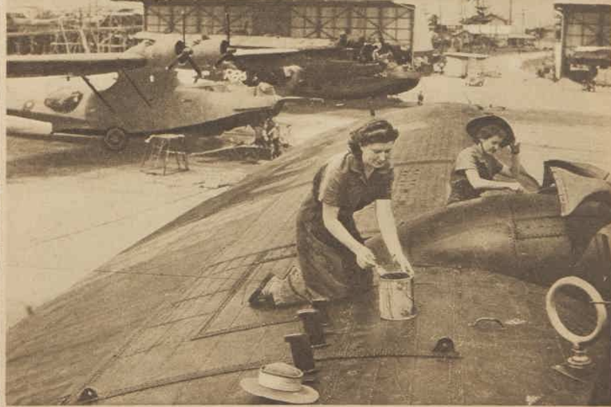
"DOPING" PATCHES on a flying-boat. Tarmac is right on the beach at this maintenance unit. Aircraft come direct from operational areas, often with bullet and shrapnel holes in fabric.
