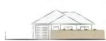
Unsuitable front fencing
