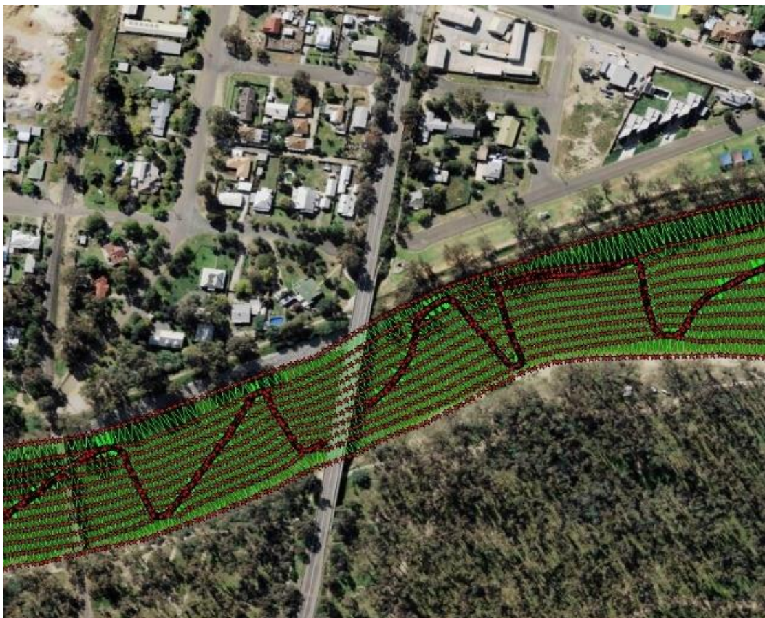
Diagram 3: River bathymetric survey at Goulburn Valley Highway Bridge
